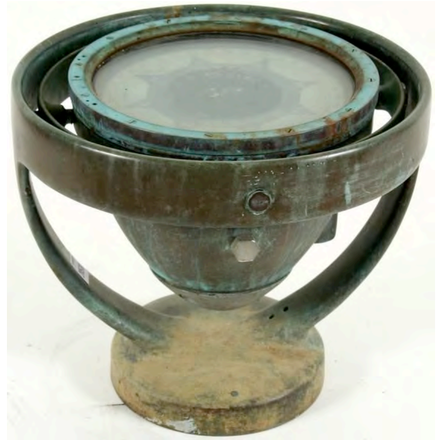
Sperry Ship Gyrocompass (1919)
