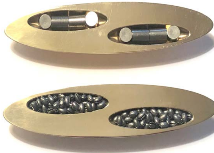
Brass \delta CELT ® with added tungsten weights (top) and lead weights (bottom)
