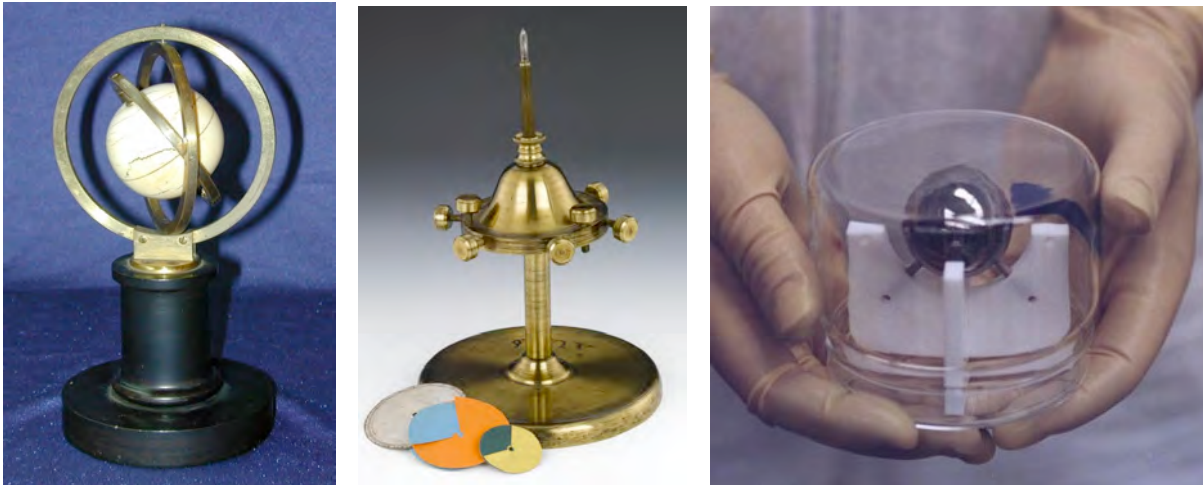
Figures 10a (l.), 10b (c.) & 10c (r.): (a) Bohnenberger Gyroscope ca. 1817 (16 cm tall); (b) James Clerk Maxwell's dynamical top 1858 (20 cm tall); (c) Gravity Probe B Gyroscope ball (~4 cm diameter).
