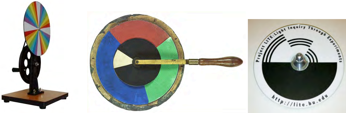
Figures 8a (l.), 8b (c.) & 8c (r.): (a) Modern version of Isaac Newton’s color mixing wheel; (b) image of James Clerk Maxwell’s color mixing top, 1855; (c) Project LITE CD Benham finger top for color, 2012.
