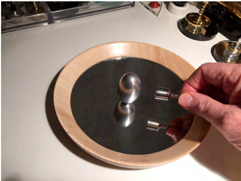
Left: Spinning Aluminum \Phi TOP Right: Spin Damped by Magnet
