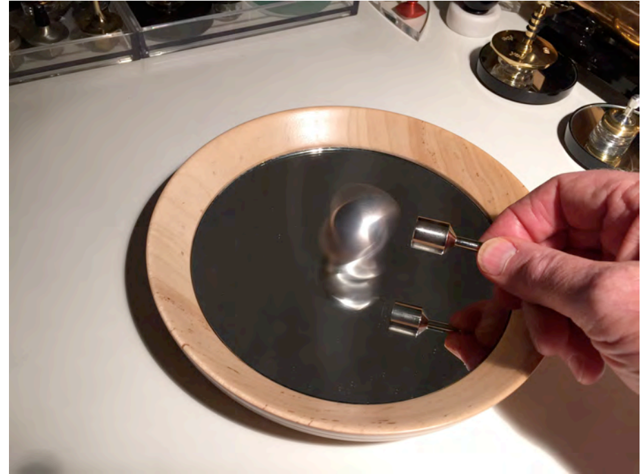
Left: Spinning Aluminum \Phi TOP Right: Spin Damped by Magnet
